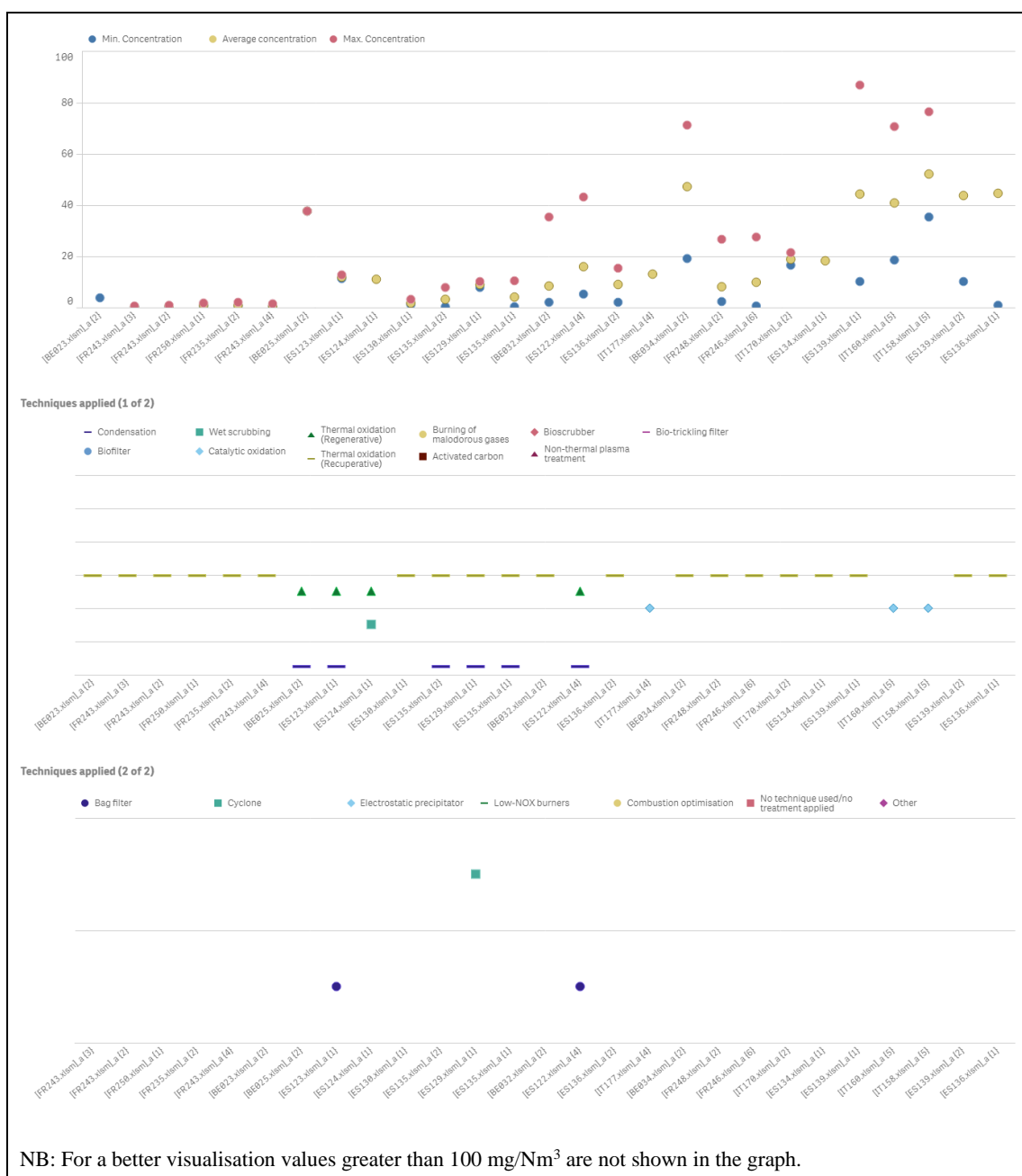
Figure 5.14: CO emissions (mg/Nm 3 ) and techniques from thermal oxidation (values corrected to 18% O 2 )
