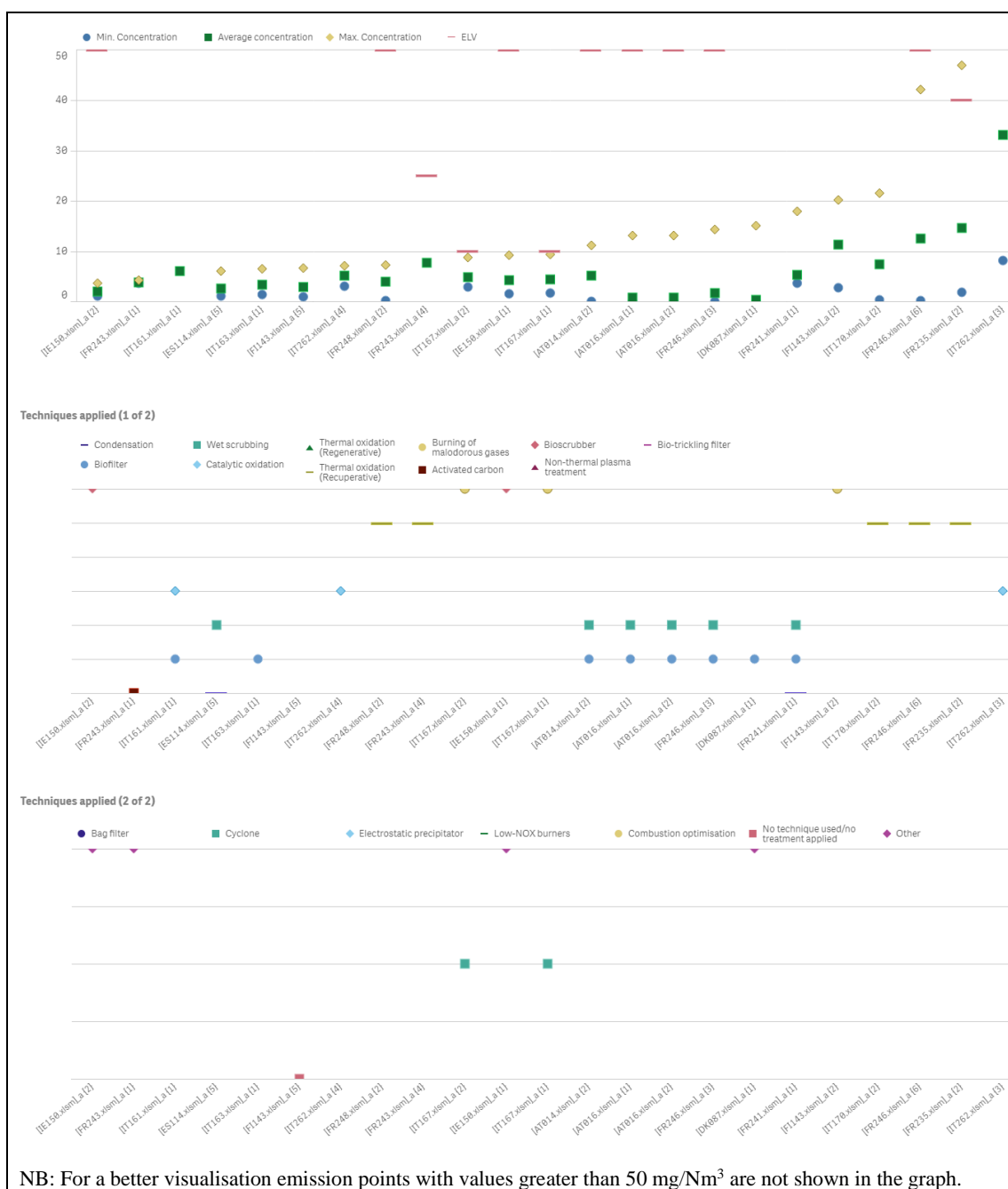
Figure 5.16: NH 3 emissions (mg/Nm 3 ) and abatement techniques from rendering, fat melting, blood and/or feather processing (Part 2 of 2)
