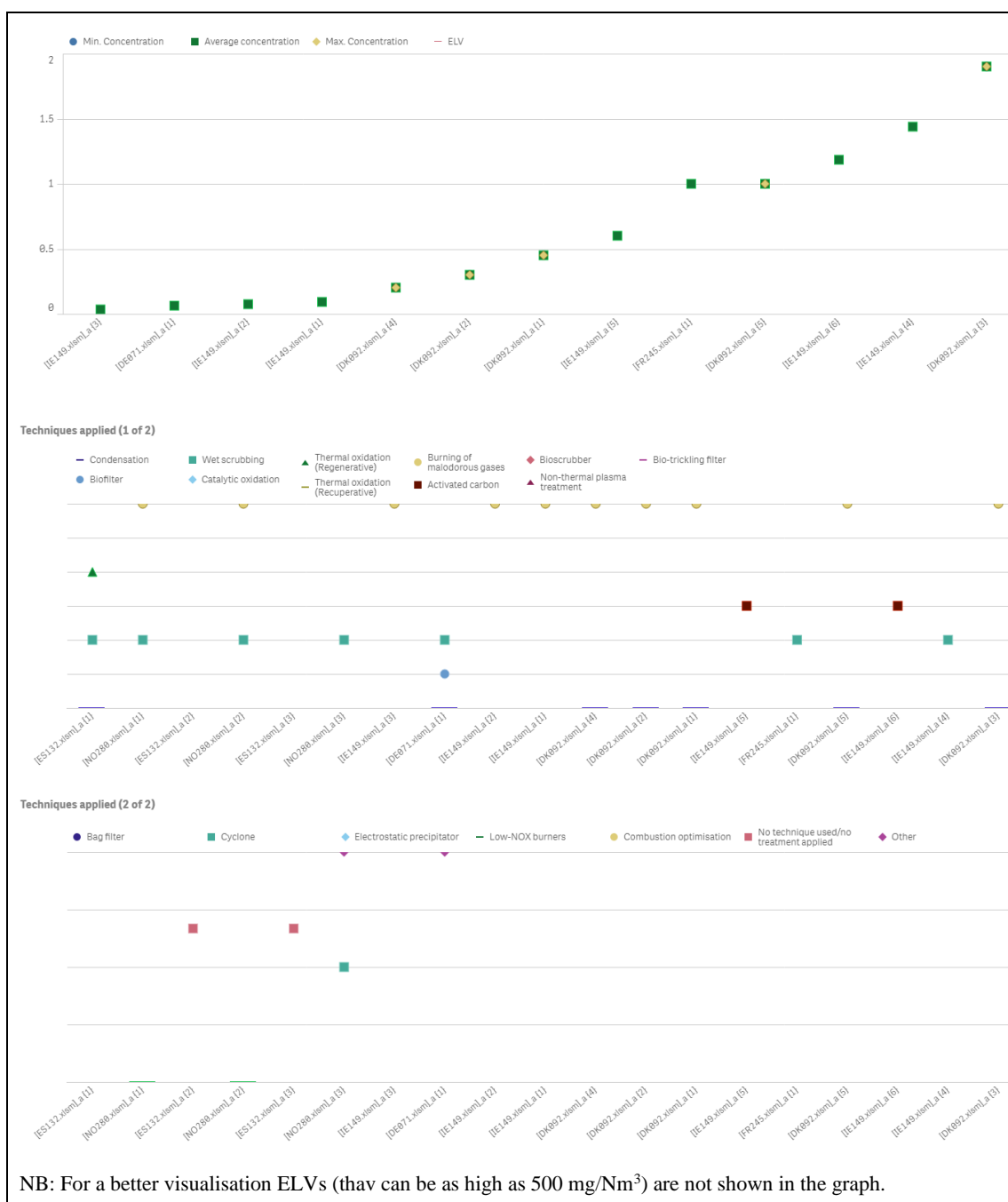
Figure 5.17: NH 3 emissions (mg/Nm 3 ) and abatement techniques from fishmeal and fish oil production
