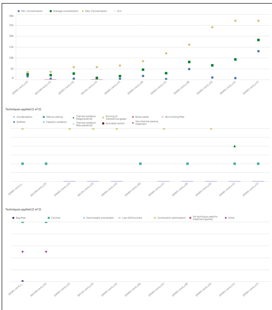
Figure 5.4: Odour emissions (ouE/Nm 3 ) and abatement techniques from fishmeal and fish oil production (Part 2 of 2)
