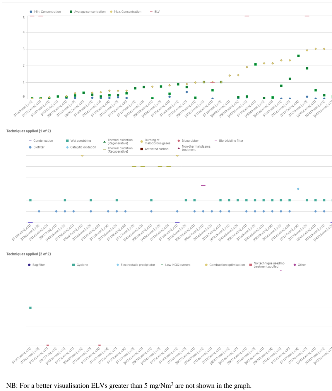
Figure 5.15: NH 3 emissions (mg/Nm 3 ) and abatement techniques from rendering, fat melting, blood and/or feather processing (Part 1 of 2)
