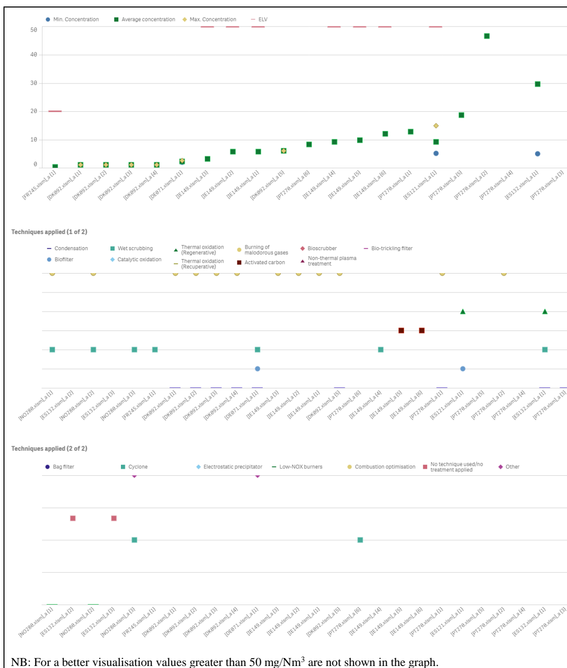
Figure 5.20: TVOC emissions (mg/Nm³) and abatement techniques from fishmeal and fish oil production
