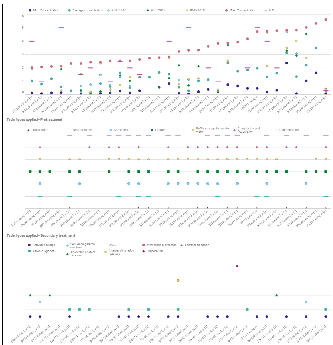
Figure 4.9: TP emissions to water (mg/l) from SA installations (direct discharges) (Part 1 to 3)
