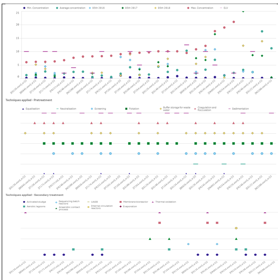
Figure 4.10: TP emissions to water (mg/l) from SA installations (direct discharges) (Part 2 to 3)
