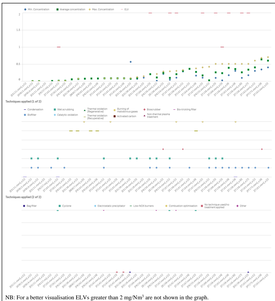
Figure 5.21: H 2 S emissions (mg/Nm 3 ) and abatement techniques from rendering, fat melting, blood and/or feather processing (Part 1 of 2)
