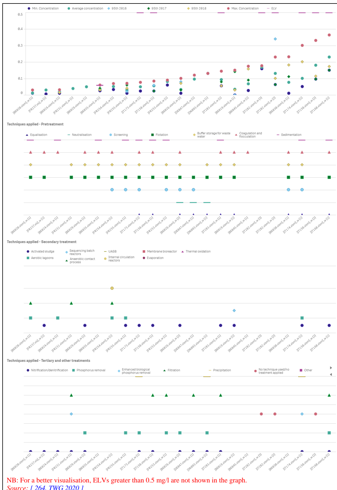
Figure 3.5: Zn emissions to water (mg/l) from slaughterhouses (direct discharges)
