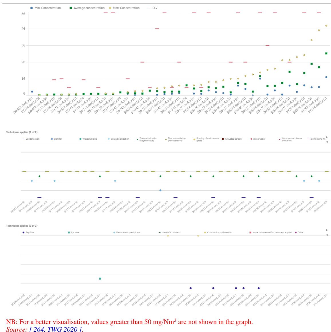
Figure 2.22: Dust emissions to air (mg/Nm 3 ) from thermal oxidation in SA installations
