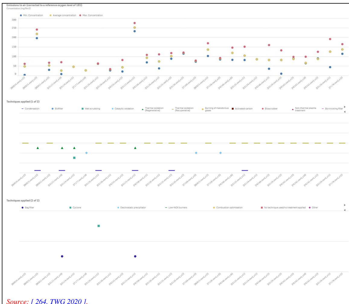
Figure 2.26: NO x emissions to air (mg/Nm 3 ) from thermal oxidation in SA installations (values corrected to 18 % O 2 )
