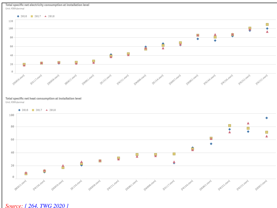
Figure 3.19: Specific electricity and heat consumption (kWh/animal) in cattle slaughterhouses (installation level)
