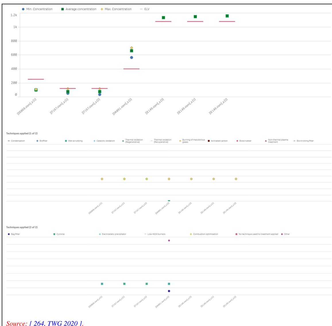
Figure 2.20: SO x emissions to air (mg/Nm 3 ) from combustion of malodorous gases including non-condensable gases in existing boilers in SA installations (Part 2 of 2)
