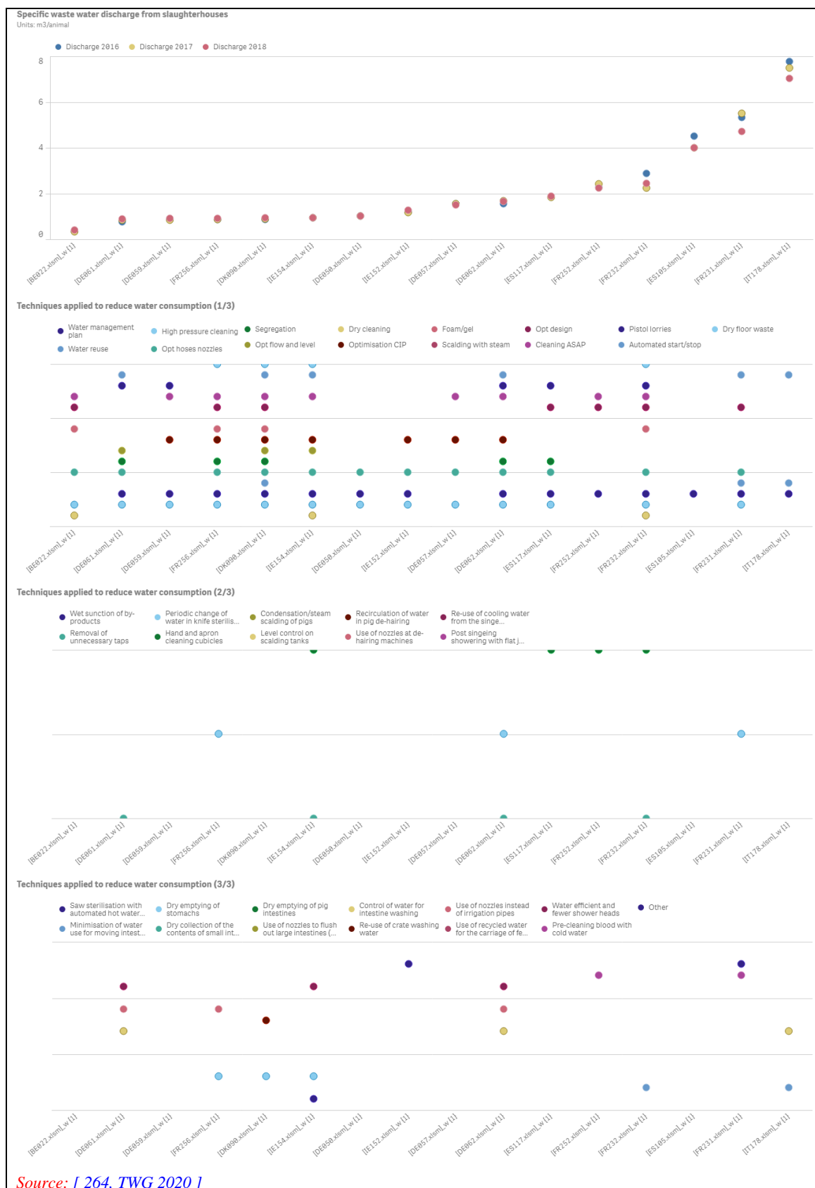
Figure 3.31: Specific waste water discharge (m 3 /animal) in cattle slaughterhouses for all types of discharges and reported techniques to reduce water consumption
