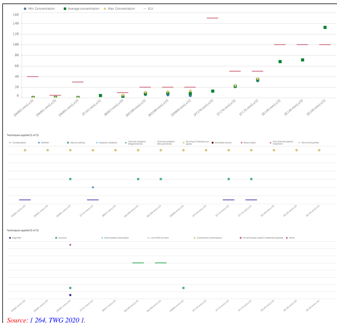
Figure 2.17: Dust emissions to air (mg/Nm 3 ) from combustion of malodorous gases including non-condensable gases in existing boilers in SA installations
